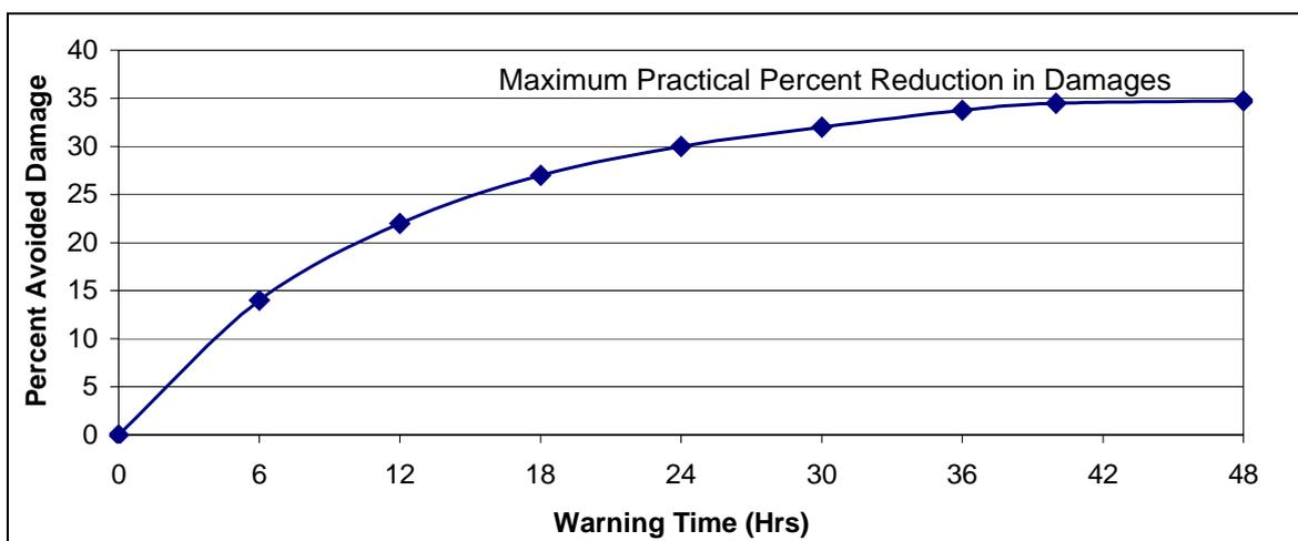
Figure 20. Day Lead time – Damages Prevented Curve (Day 1970).
