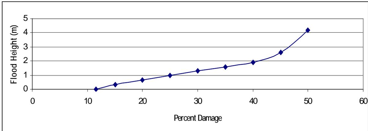
Figure 8. Stage-damage curve for a one-story home (USACE 1995).
