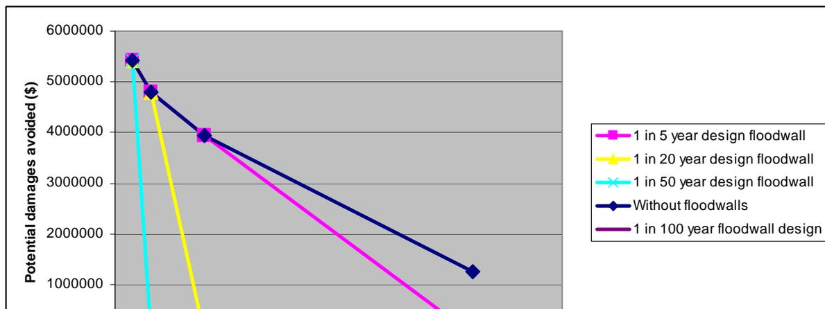
Figure 16. Plot of avoided damages from the construction of floodwalls.
