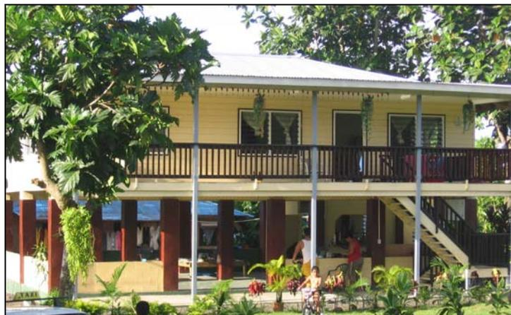
*Figure 23. Living space of home is elevated well above ground level.*
