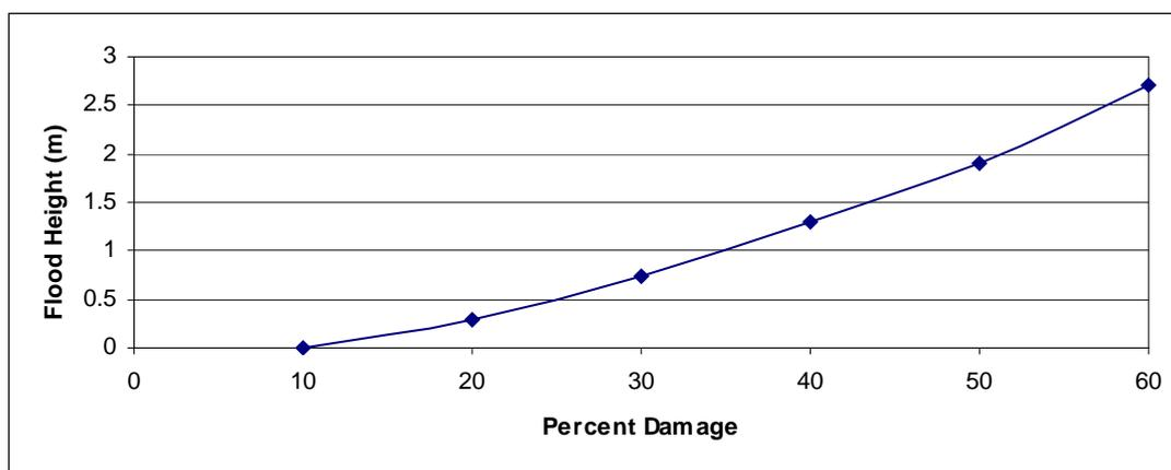
Figure 9. Stage-damage curve for household contents (USACE, 1995).
