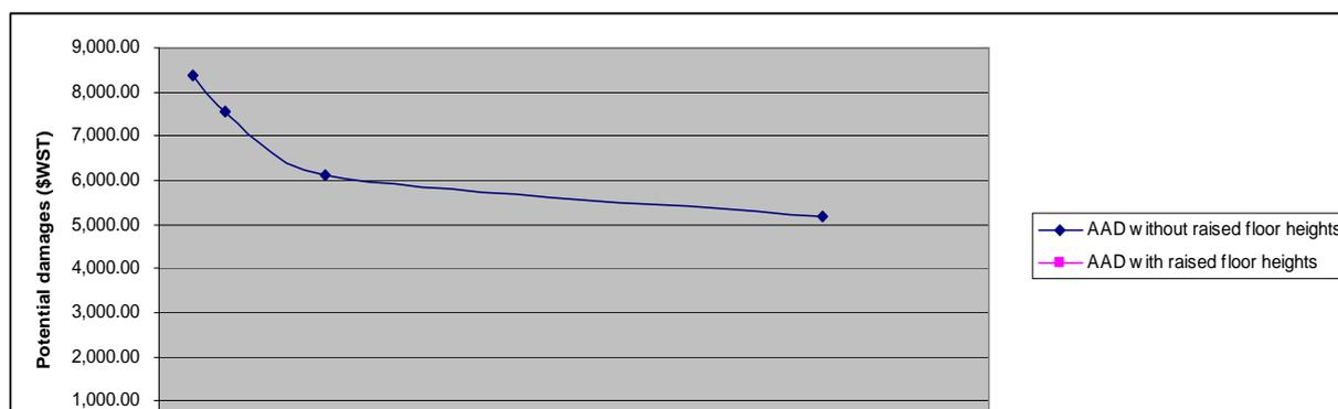
Figure 24. Plot of avoided damages from raising the floor height of a home.
