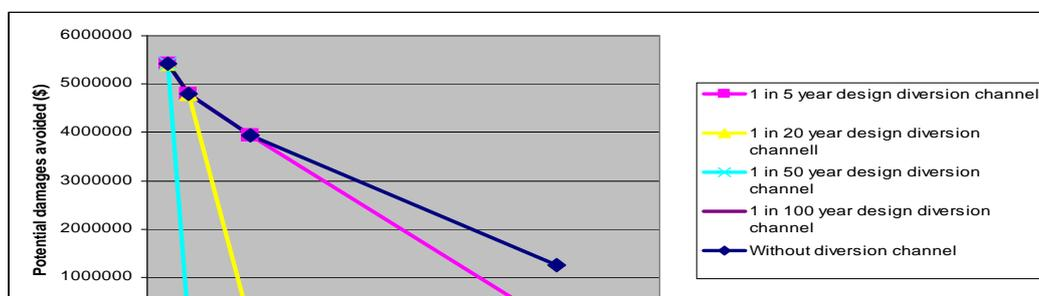
**Figure 19.** Plot of avoided damages from the construction of a diversion channel.**Table 40.** Annual average damage avoided by constructing diversion channels.
