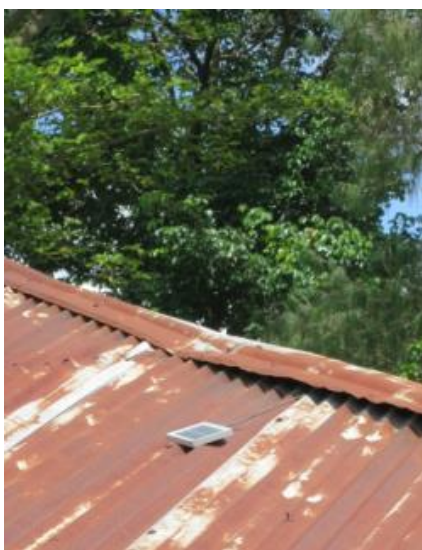
Figure 27 Two households permanently leave the solar panel of the S250 on the roof, which not only increases the risk of theft, but also that of damage.
