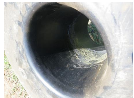
Figure 22 A leak at the inside seam of a Q Drum is sealed by melted plastic.
