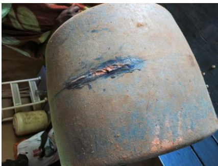
Figure 23 One household fixed the leak by applying melted plastic to the leak.
