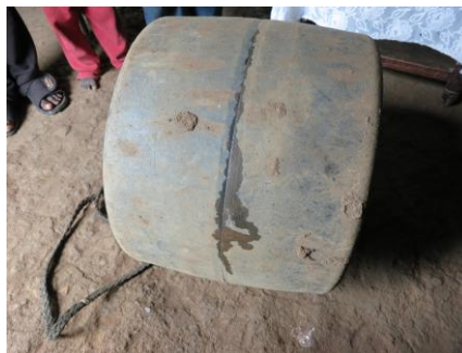
Figure 24 Water leaks from the outer seam of a Q Drum.
